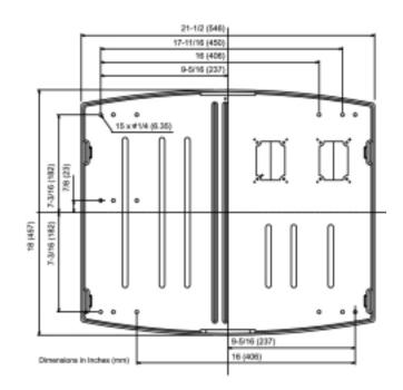
Figure 7 – Wall Baffle Mounting Holes
